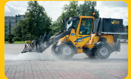
Water tank for high-pressure washing
